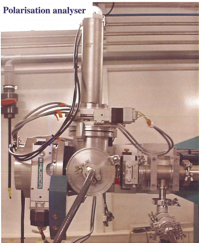
The polarisation analyser, shown in-situ on the 2-theta arm, has been operational for more than a year now and seen service with several users.
