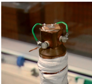
Fig. 13: Example of PZT sample mounted on the XMaS cryostat. The bottom electrode is mounted on a sapphire plate.
