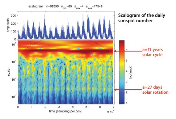
**Cone of influence:** defined as the *e*-folding time for the autocorrelation of wavelet power at each scale.
