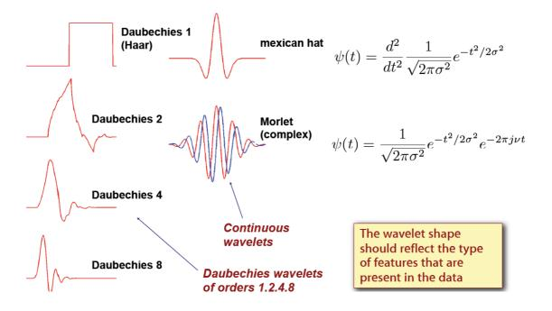
'order' of a filter refers to the degree of the approximating polynomial in frequency space- must exceed that of the signal.
