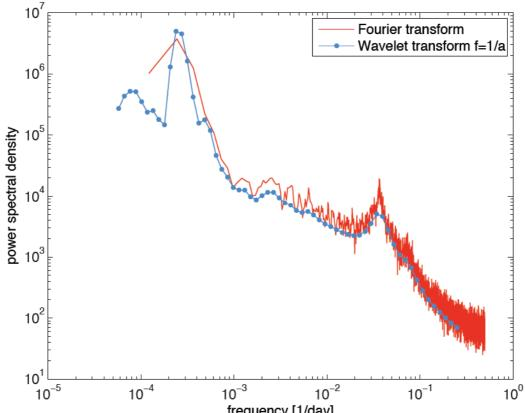
frequency [1/dav] Note the self- similar nature of the scaling/dilation of the wavelet transform results in uniform binning in log space of frequency (Fourier has uniform binning in linear frequency space).
