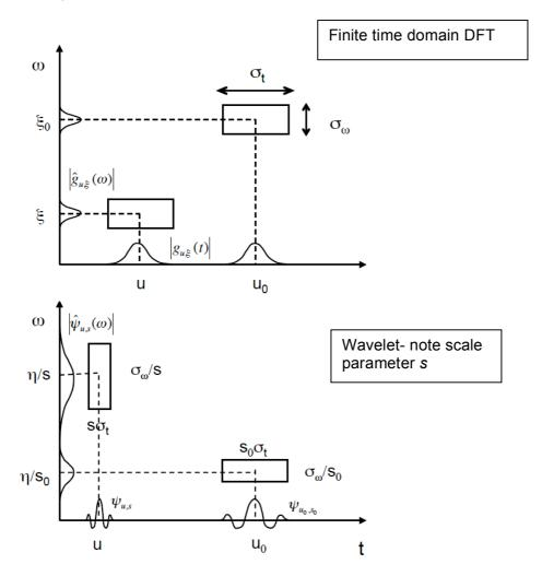
So at its simplest, a wavelet transform is simply a collection of windowed band pass filters applied to the Fourier transform- and this is how wavelet transforms are often computed (as in Matlab). However we will want to impose some desirable properties, invertability (orthogonality) and completeness.
