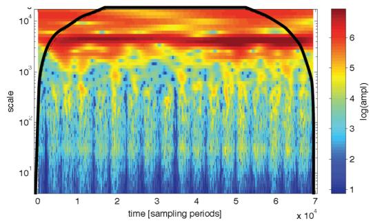
**Estimate of Power Spectral Density (PSD):** in the same manner as integrating a Fourier spectrogram across time to obtain an averaged PSD one can integrate the wavelet scaleogram across time:
