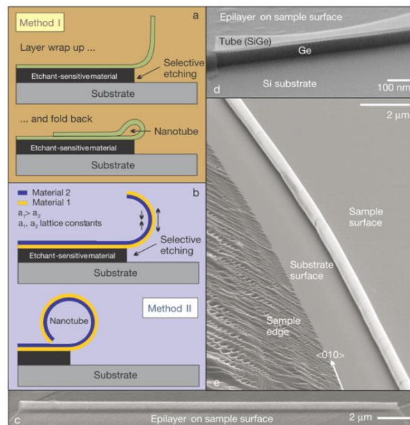
Figure 5.14: Nanotube formation (a) method I (b) method II (c) 12\mu\text{m} long nanotube from method I (d) 50\text{nm} diameter nanotube from method I (e) 12\mu\text{m} long nanotube from method
