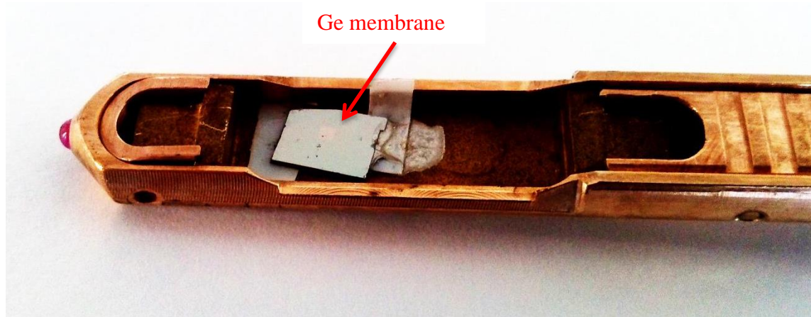
Figure 6-10 - Modified TEM Sample holder containing Ge membrane. The membrane is faintly visible due to optical transparency.
