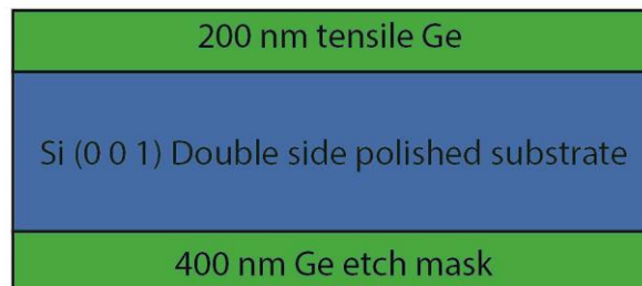
Figure 6-2 - Schematic diagram of Ge growth for thin membrane
