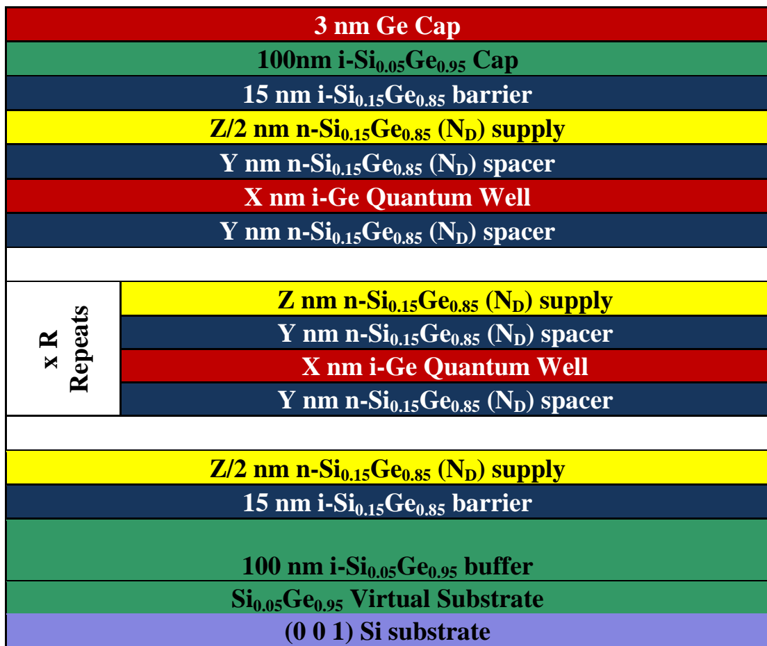
Figure 5-5 - Schematic diagram of FTIR layer structure
