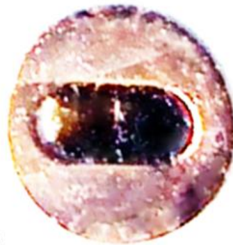
Figure 3-26 – Ground, polished and ion milled sample with copper support ring glued to surface
