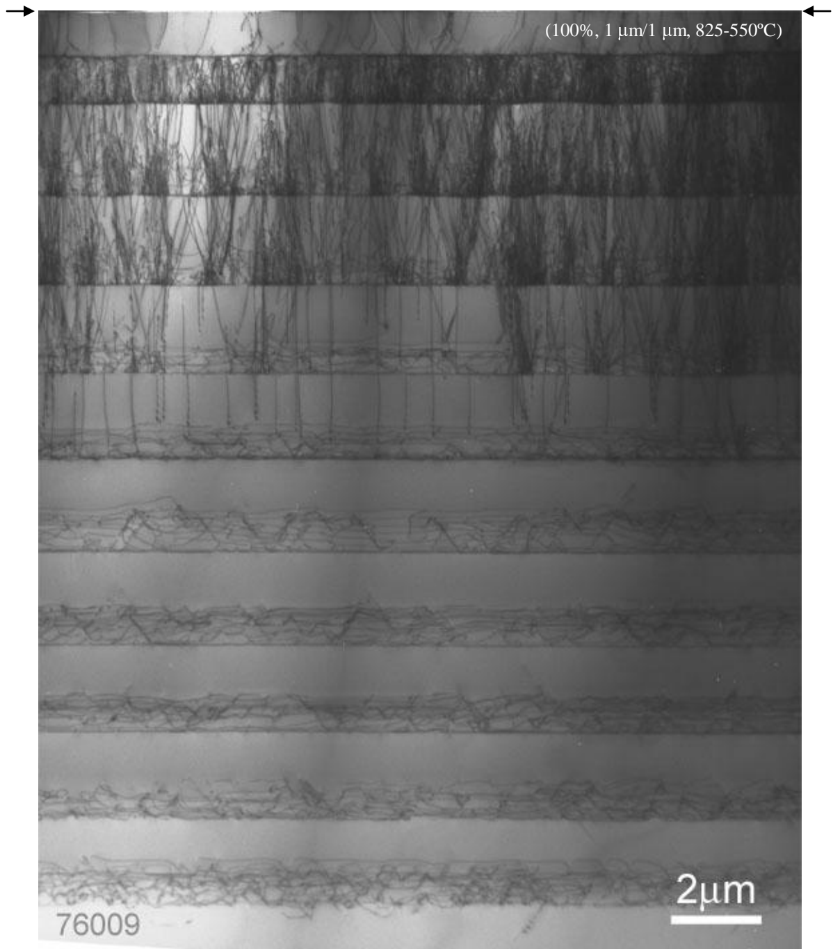
Figure 6.8 – Cross-sectional TEM image of sample 76009 in the (220) two beam diffraction condition highlighting dislocations within the structure. Arrows indicate the structures surface.
