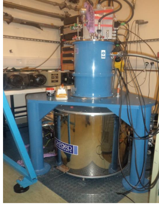
Figure 3.8 Image of 300 mK, 12 T cryomagnetic system (Heliox)
