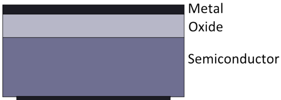
Figure 2.1: Schematic of a Metal-Oxide-Semiconductor capacitor with the back contact present. The semiconductor can be n- or p-type. The metal gate act as a gate for the device.
