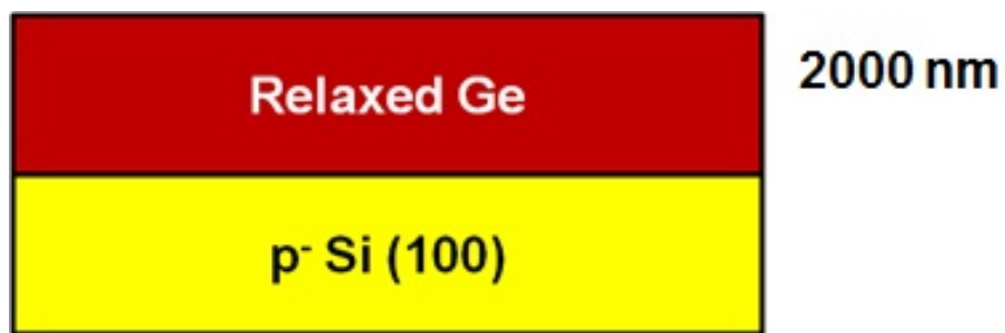
Figure 4.1: Schematic diagram of the structures for relaxed germanium layers. The rGe layers consisted of a thick Ge layer grown directly on a Si substrate.
