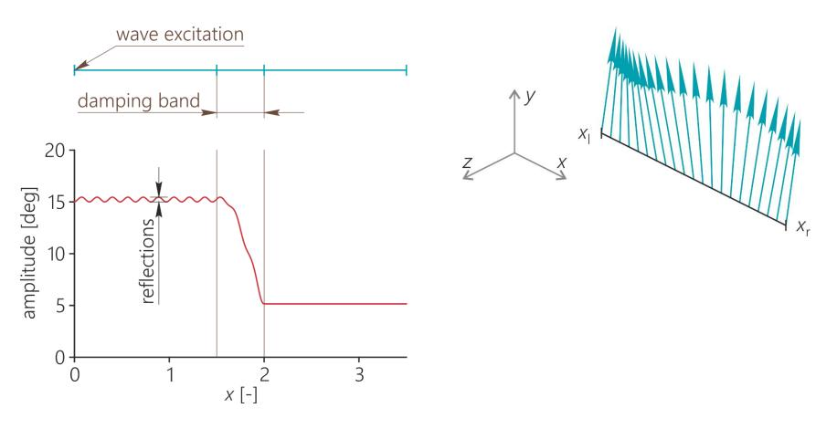
width of the damping band determines the scale of reflections from it
