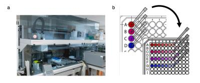
Figure 1: Liquid handling system a) The Tecan platform used to prepare and measure plates. b) Compounds, supplied by the client in 96 well plates, are transfered onto 384 well plates and then inoculated
