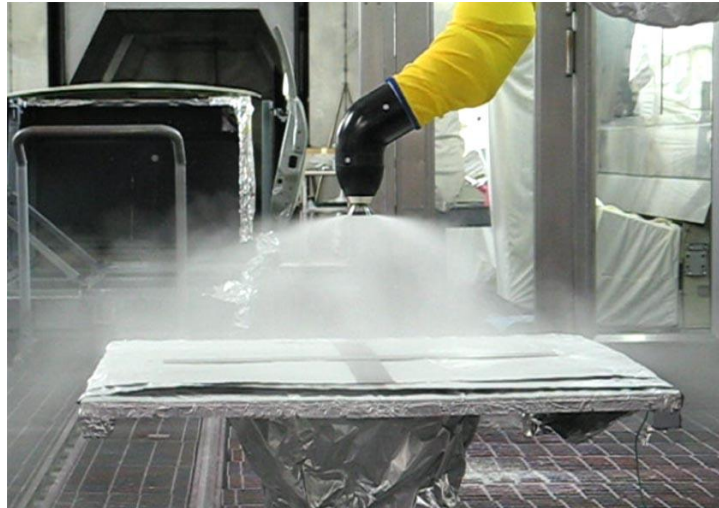
Figure 4.2: Photograph of one of the experiments. The rotating bell is at the end of the robot arm spraying paint onto the target square plate.
