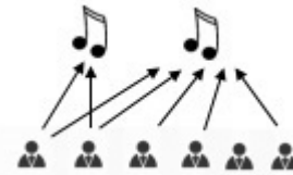
Figure 2. A schematic example of a network with tracks and users. There are only edges between tracks and users, not between users and users or tracks and tracks.
