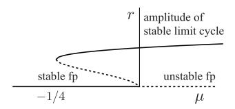
At  $\mu=0$  there is a **sub-critical Hopf bifurcation**. The system also exhibits hysteresis; once large amplitude oscillations have begun they cannot be turned off by bringing  $\mu$  back to zero. In fact they persist until  $\mu=-1/4$  where the stable and unstable cycles collide and annihilate in a **saddle-node bifurcation** of limit cycles.
