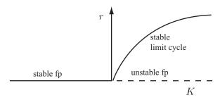
This is an example of a **super-critical Hopf bifurcation**. Since an arbitrarily small perturbation of the origin will produce a self-sustained oscillation the system is said to exhibit a **soft excitation**.
