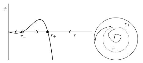
For  $\mu <$  0 there exists a stable fixed point at the origin, an unstable limit cycle at  $r=r_-$  and a stable limit cycle at  $r=r_+$  where
