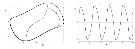
The van der Pol equation has a unique, stable limit cycle for each  $\mu > 0$ .
