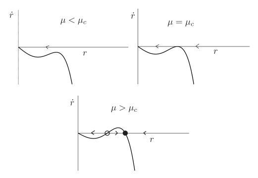
When the system passes through the sub-critical Hopf bifurcation it jumps from the fixed point to a large amplitude oscillation — termed a **hard excitation**. This is potentially dangerous in engineering applications.
