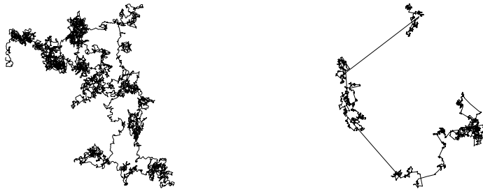
Fig. 17. Trajectory in 2D space of a particle with Brownian motion (left) and Lévy random walk (right).
