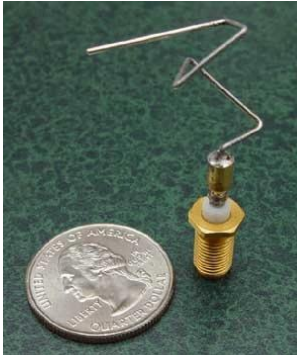
The 2006 NASA ST5 "evolved" spacecraft antenna.
