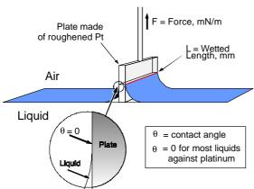
The Wilhelmy plate method is the most prominent method for measuring equilibrium surface tensions of liquid samples. A small platinum coupon is attached to a force-measuring sensor and precisely dipped into a liquid and withdrawn to the point where the bottom edge of the coupon is exactly parallel with the surface of the bulk fluid itself. At this point, the surface tension is related to the force exerted by the liquid wetting it by the following equation:
