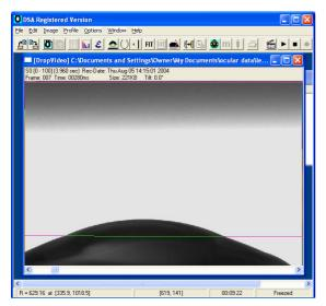
Although it may be difficult to see with the straight baseline in the image, the drop does exist in the image above. The drop edges are approximately where the baseline in the image crosses the sample. A simple circle fit was used to provide contact angle values. The drop shape above looks reasonable and gives reasonable data for the sample.
