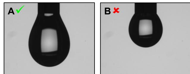
Fig. 4: Adequately (A) and inadequately (B) deformed pendant drops.
