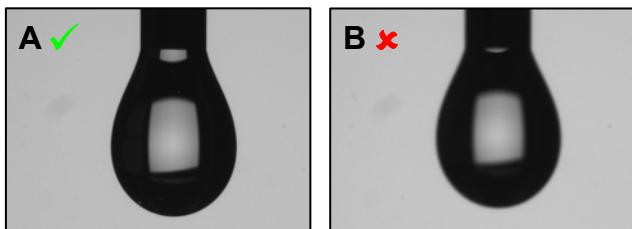
Fig. 6: Correct (A) and incorrect (B) focus setting.
