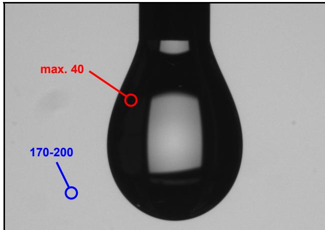
Fig. 8: Gray level values of the drop and surrounding phase under optimal illumination.
