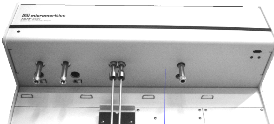
Manifold Probe Hole (to the left of the analysis port)
