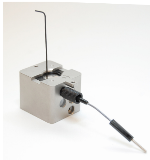
The reference electrode (yellow color in graph) mounted correctly, so that it barely protrudes into the flow channel and does not disturb the flow. The distance to the working electrode (sensor surface) is 5 mm.
