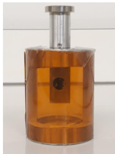
Figure 1: OpMetBat cell developed for transmission and grazing incidence XRD measurements at XMaS.
