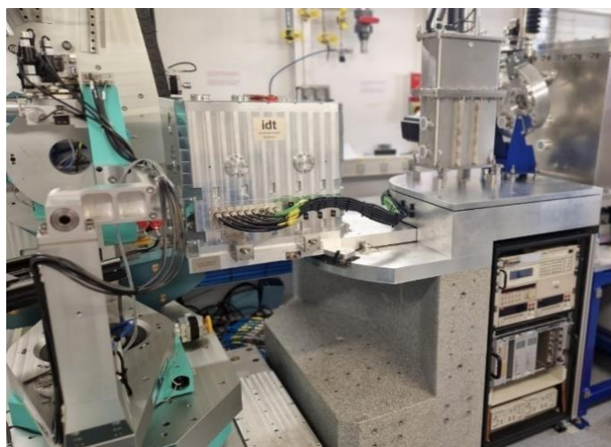
Figure 2: The IDT KB mirror system installed on the beamline.
