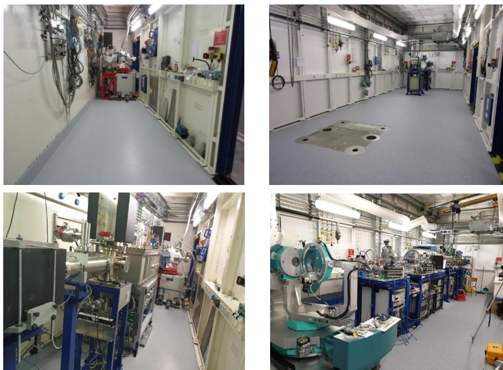
Figure 12: Optics hutch (left) and experimental cabin (right) before (top) and after (bottom) the extensive rebuild of the beamline.
