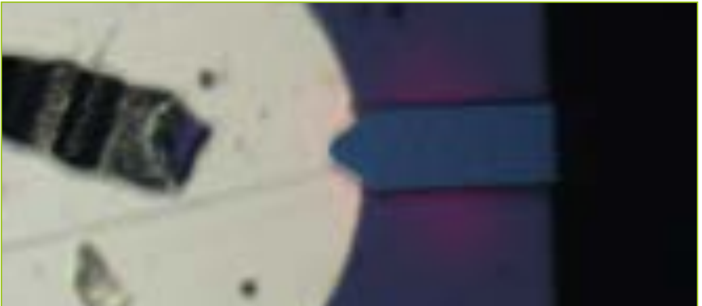
Figure 4 – PZT sample with a circular top electrode and AFM probe in contact with the electrode
