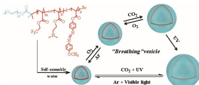
Scheme 6. The structure of the triblock copolymer (PEG- b -P(DMAEMA- co -TFEMA)- b -PMEPPMA) showing self-assembly and its tri- stimuli-responsive 'breathing' behaviour. 64 Adapted from P. Theato et al , Macromol. Rapid Commun. , 2018, 39 , 6.
