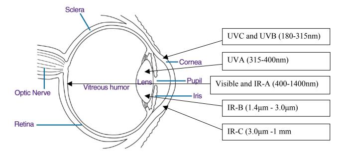
NB Short pulsed high peak-power laser beams are particularly hazardous to the eye, especially at wavelengths that reach the retina, as they deliver a lot of energy in a short period of time that can cause irreversible damage. Near infra-red lasers are also particularly hazardous because you can't see the beam but it could be focused on the retina and you would only be aware of it after damage has been caused.
