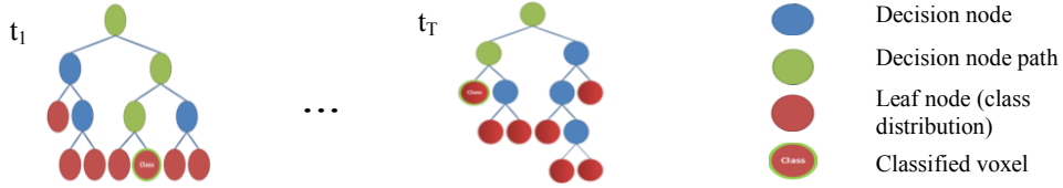
Fig. 1. Random forests which contain T decision trees. Decision is made as a combination of class distribution (red circles with green outline) from every tree ( t_i ).
