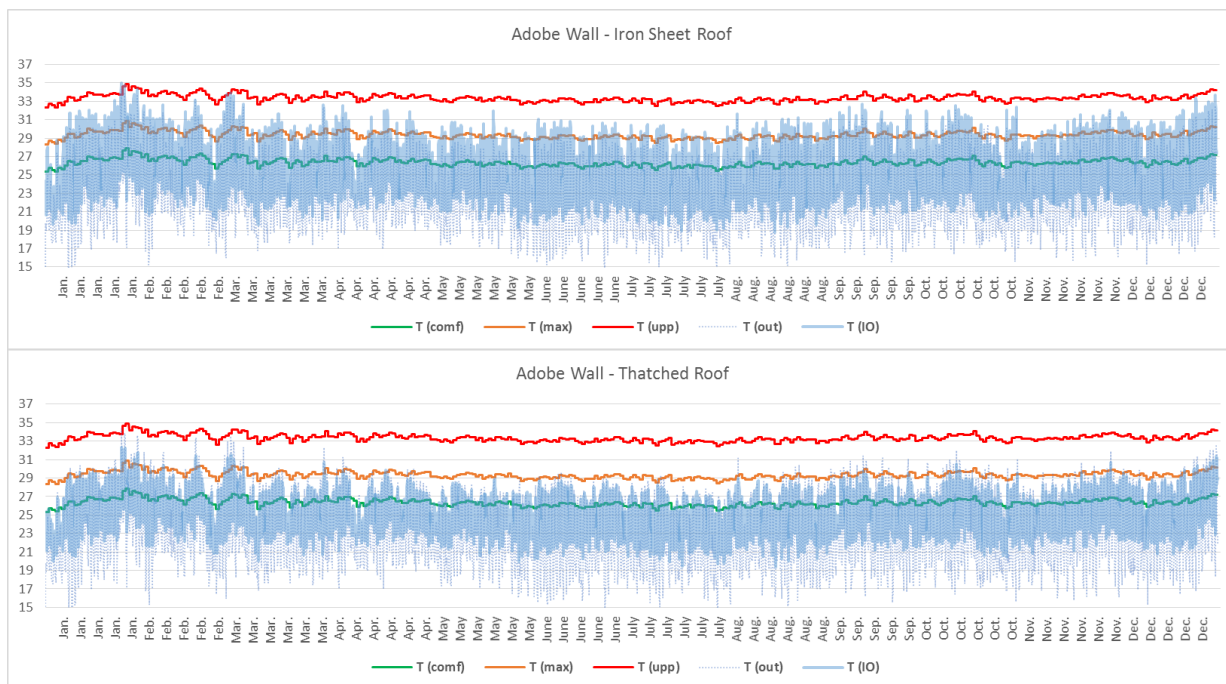
Figure 3: Thermal comfort condition for adobe walls with iron sheet (top) and thatched roofs (bottom).
