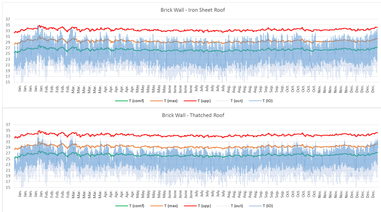
Figure 4: Thermal comfort condition for brick walls with iron sheet (top) and thatched roofs (bottom).
