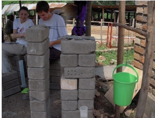
Figure 9 - Photograph of Stiffness Test Rig
