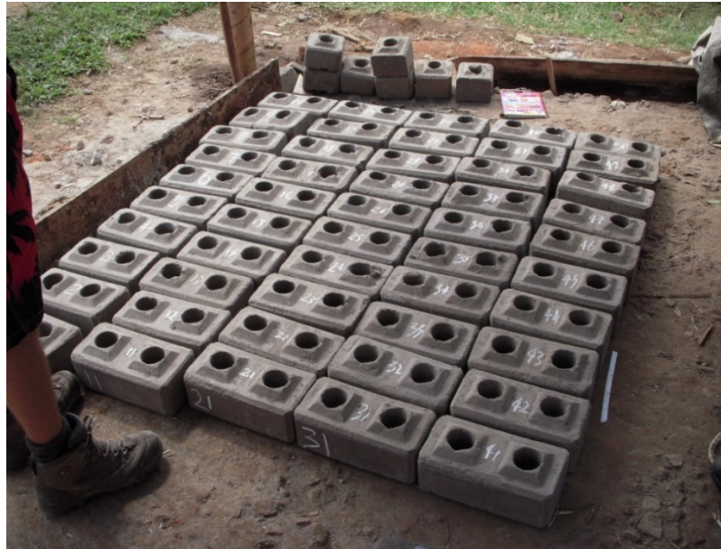
Figure 2 – Sample of 50 stabilised soil bricks used in tests.
