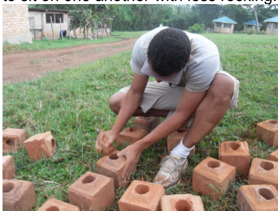
Figure 7 Rasping the bricks
