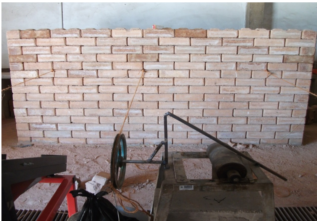
Figure 2: Bespoke Pulley System for Lateral Load Application of straight wall
