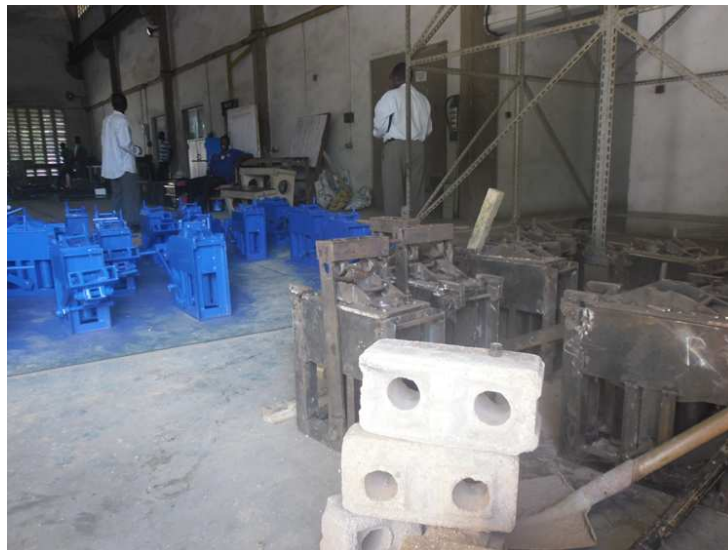
Plate 6.2: NHBRA Interlocking Brick Press Machine manufacturing yard
