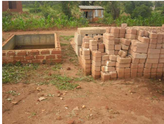
Plate 6.1: Locally produced interlocking bricks (right) and burnt bricks (left) in Morogoro(using the same raw material, suitable soil)
