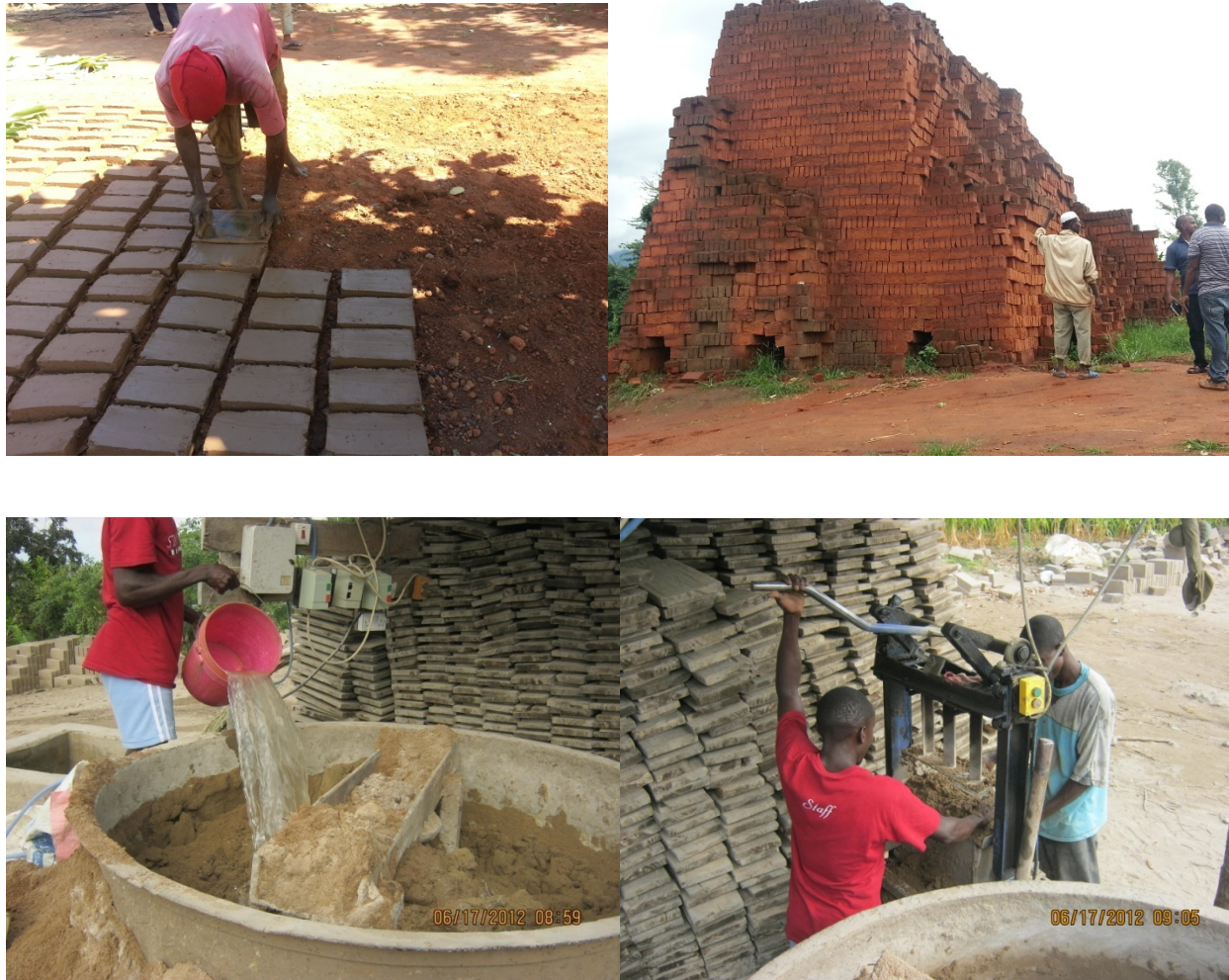
Plate 3: Production of adobe (upper left); burnt bricks (upper right); sand cement block (lower left and right)
