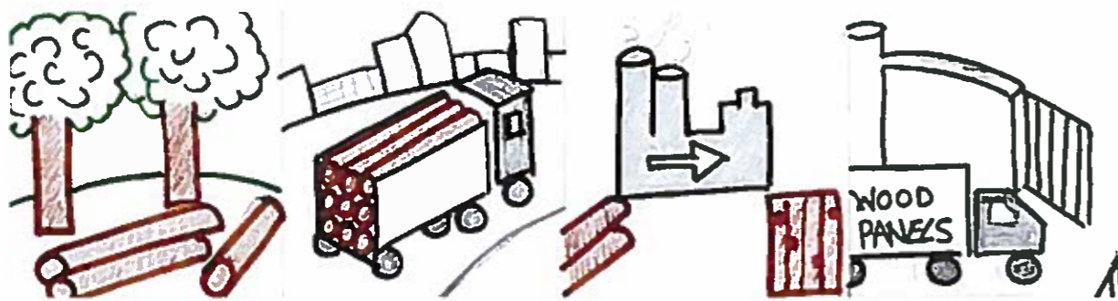
Figure.8. Illustration of activities contributing to Embodied Energy in the cradle to gate energy analysis (Author)
