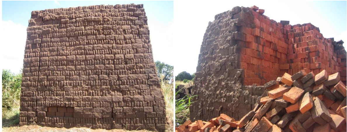
Figure 4: Bricks within 300mm of the clamp kiln's surfaces have a very low quality (Tanzania).
