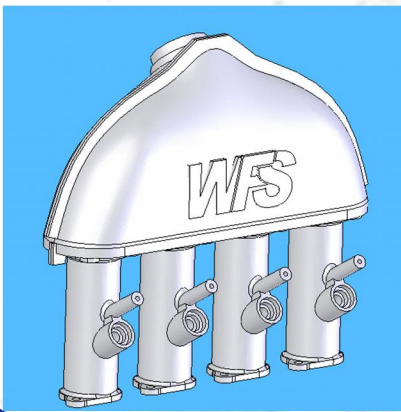
A CAD design of the air intake system for our new 2007 car.
