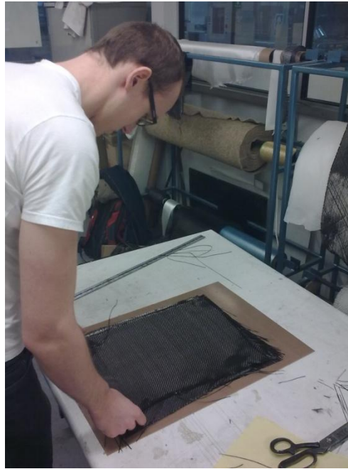
Figure 22 - Placing carbon fibre fabric on tool
