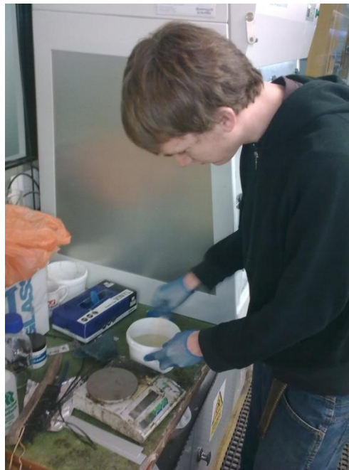
Figure 27 - Mixing of EP522 and H522
