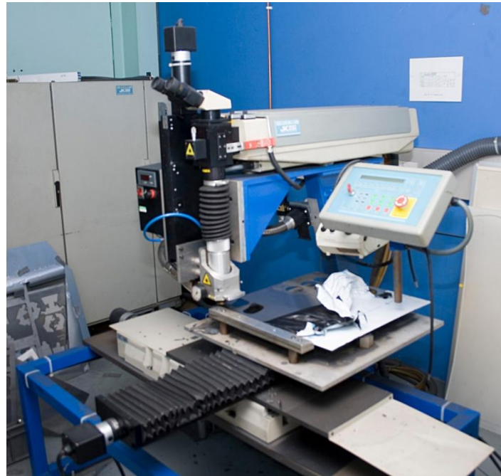
Figure 35 - Lumonics JK 701 Yag Laser
