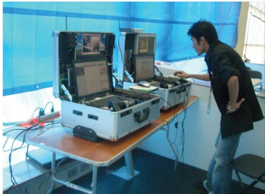
Figure 4 – An example of a tele-operated control system using laptops and hand held controllers
