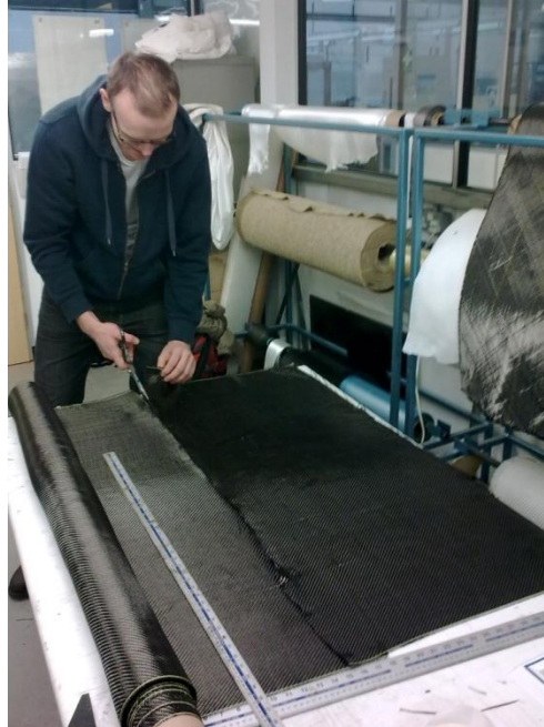
Figure 21 - Cutting carbon fibre fabric
