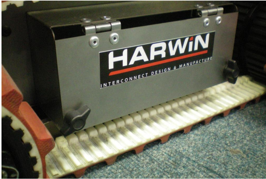
Figure 16 - Closed Battery Pack
