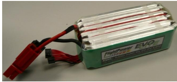
Figure 43 – Old 24V LiPo Batteries
