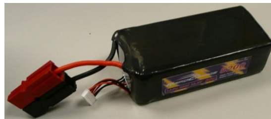
Figure 44 – New 24V LiPo Batteries (1)
