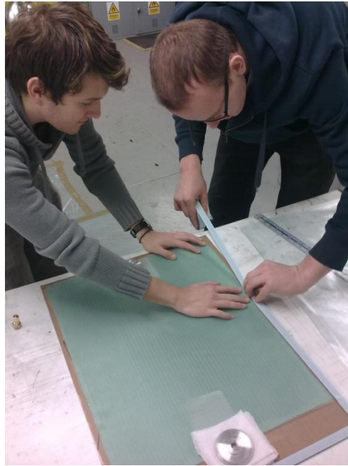
Figure 24 - Sealant tape being placed around the edges of the tool
