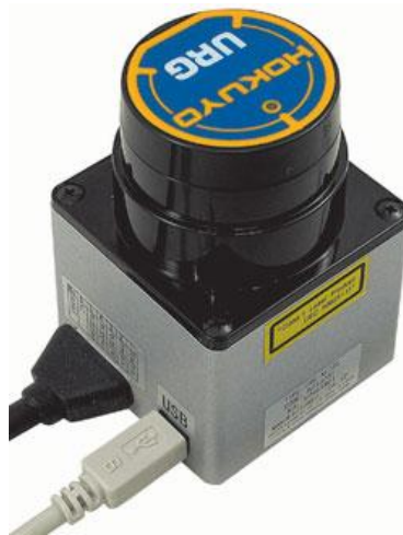
Figure 79- The laser scanner that was used on both the autonomous and tele-operated platforms
