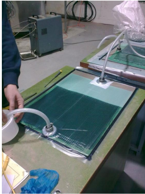
Figure 28 - Sucking mixture into carbon fibre sandwich
