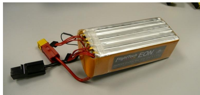
Figure 45 – New 24V LiPo Batteries (2)
