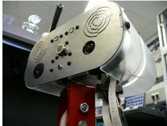
Figure 85 - Servo motor and electronic wires head cover cut-outs
