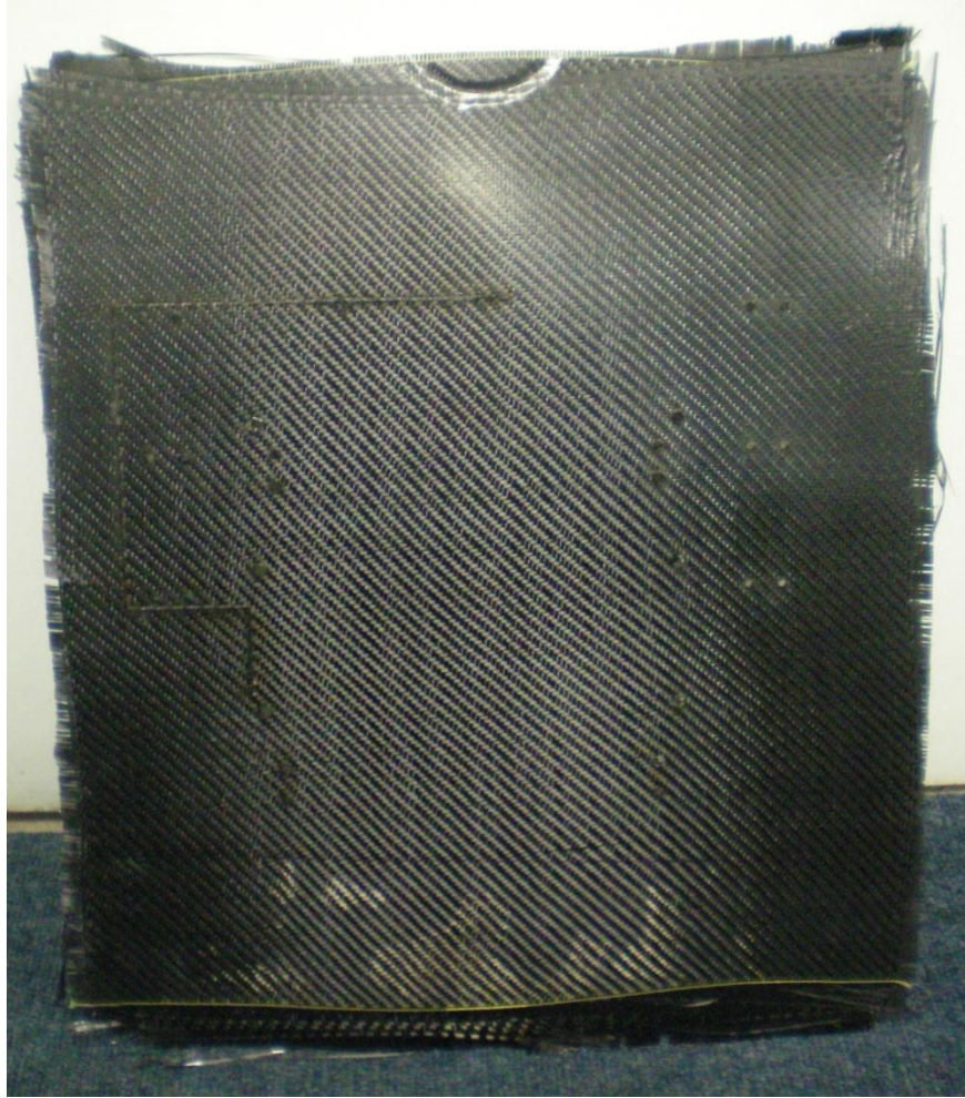
Figure 32 - Uncompleted laser cut carbon fibre panel
