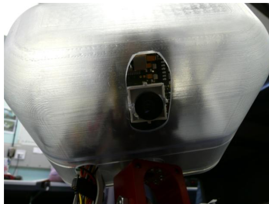
Figure 84 - Rear camera head cover cut-out
