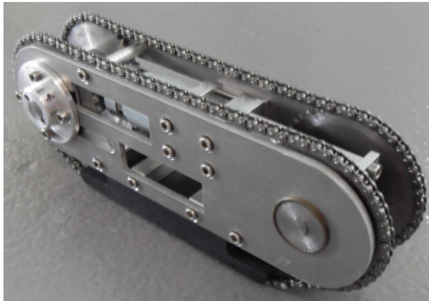
Figure 39: Manufactured & Assembled Track Unit (With Tensioning Block)
