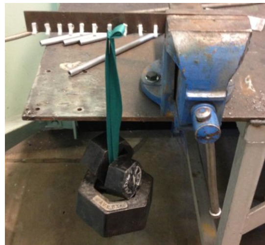
Figure 43: 88.29N Applied to Bonded Aluminium L Section and Withstood
