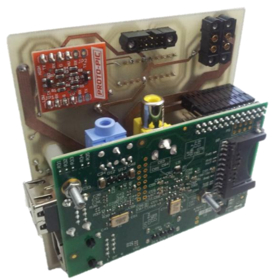
Figure 141: Arm Power Board Mounted to Raspberry Pi
