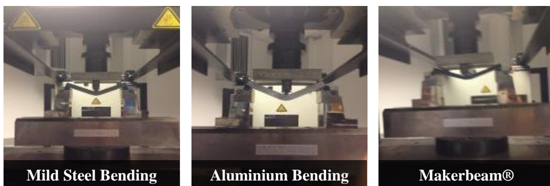
Figure 12 – Bending tests on mild steel, aluminium and MakerBeam ®
