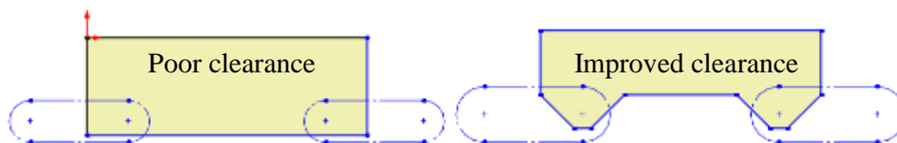
Figure 11 – Chassis clearance improvement
