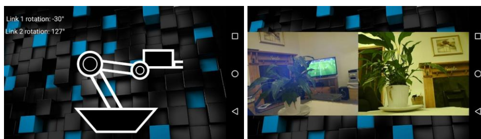
Figure 44: The ATLAS App – Robot Arm Inverse Kinematics (Left) and Video Feed (Right)
