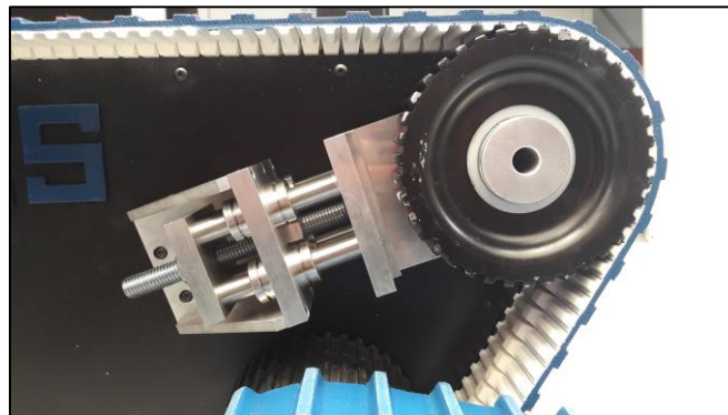
Figure 24: Static Tensioning system upon attachment to the chassis
