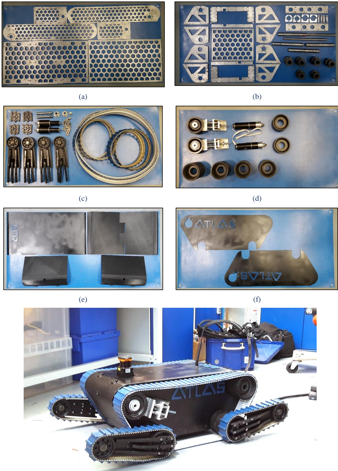
Figure 47: ATLAS Final Assembly (a) Main Chassis, (b) Lower Chassis & Suspension, (c) Flippers and Tracks, (d) Tensioning and Drivetrain, (e) Cladding Plates (f) Side Cladding & Logo
