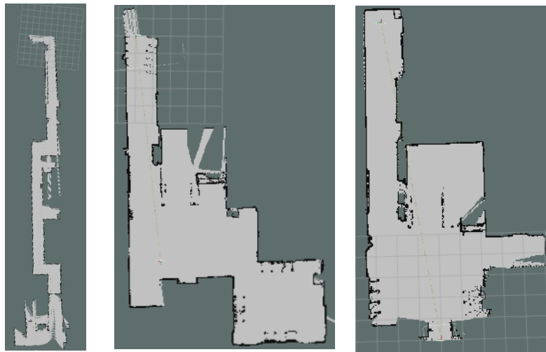
Figure 54: LiDAR maps of Warwick's engineering department (from left to right): second floor, third, floor, fourth floor
