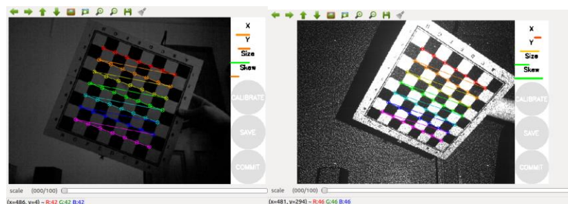
Figure 51: Calibrating the Kinect
