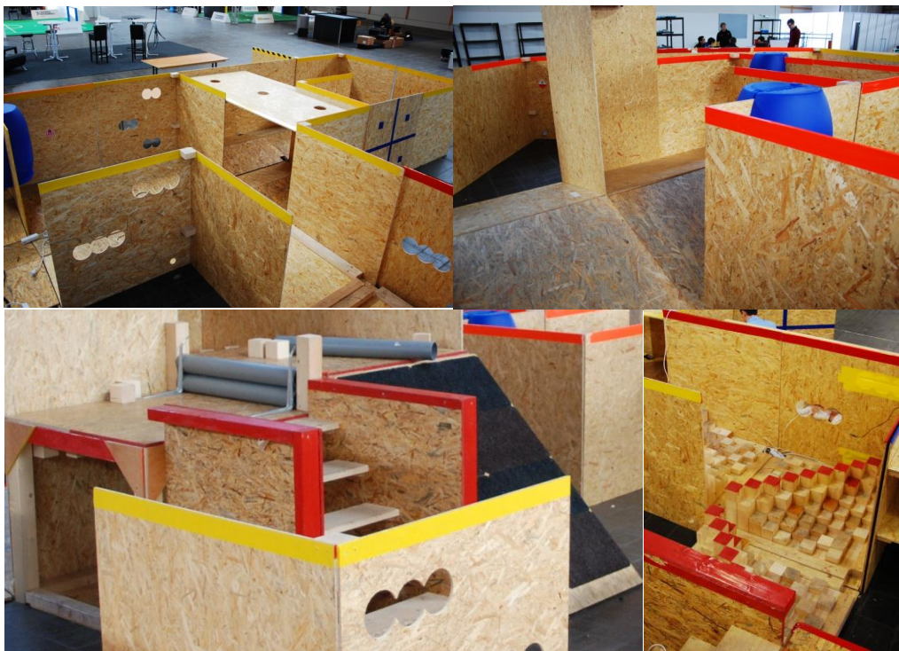
Figure 7: a) The Yellow arena b) The Orange Arena c) The red arena ramp and stairs d) The red arena stepfield
