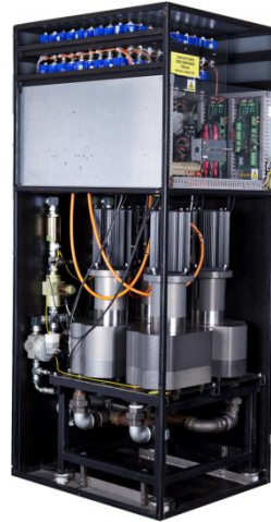
(a) Parallel scroll expanders combined with supercapacitor array for high power applications
