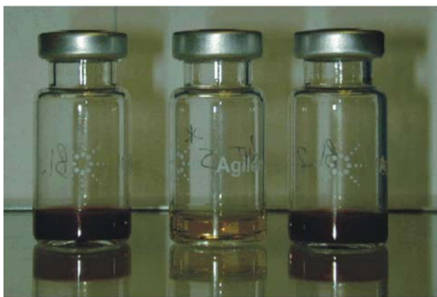
Fig. 2: Photograph of 10 ml vials with aluminium crimped cap and PTFE/silicone septum and 1.5 ml aliquots of blood or blank media.
