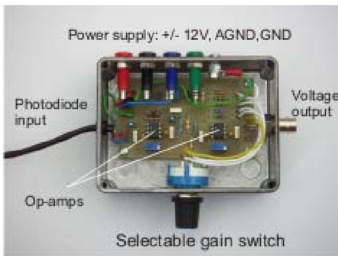
Fig. 7: Photograph of amplifier circuitry.
