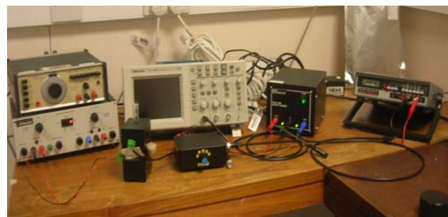
Fig. 11: Prototype optical biosensor system for immunoassay application showing DC LED power supply, digital scope, circuit DC supply ( \pm 12 V), and DVM (from left to right).
