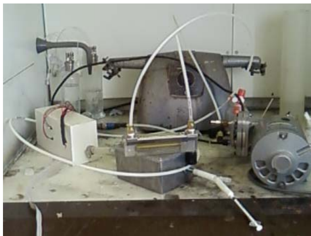
Figure 5 Experimental arrangement used to measure the odour pulses within the artificial nasal cavity
