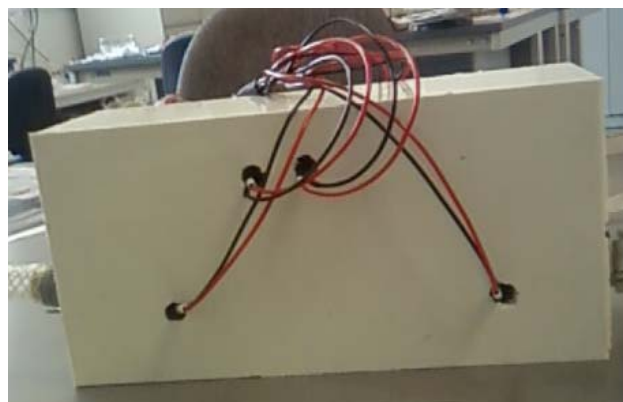
Figure 6 Photograph of 3-D model of nasal cavity with six embedded odour sensors
