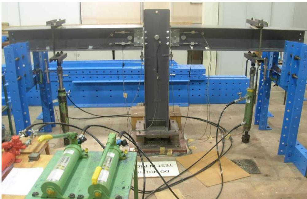
Fig. 2. General test arrangement for major-axis beam-to-column joint Wmj254\_3M16\_FC1-4.
