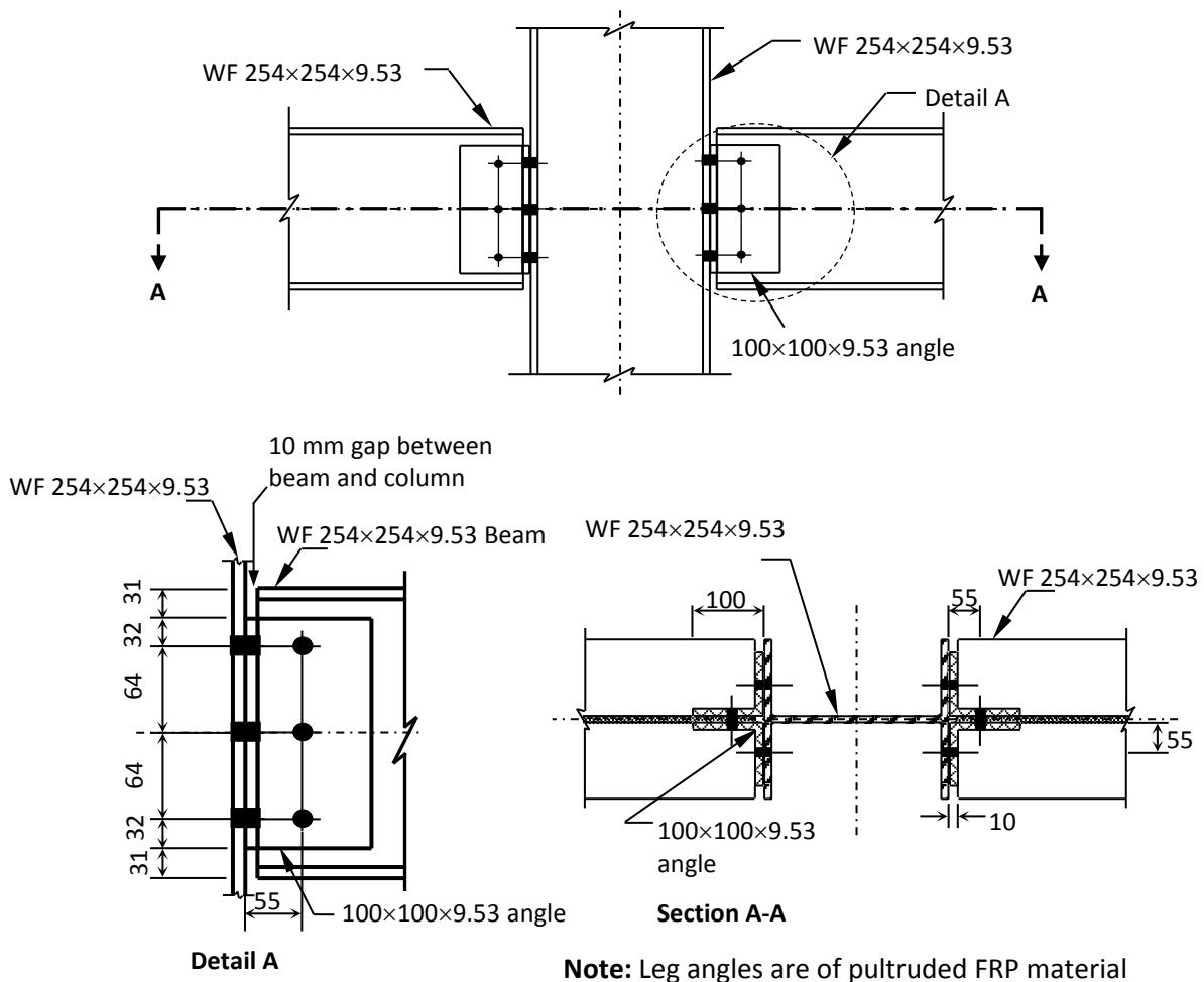
Fig. 4. Connection details for nominally pinned beam-to-column joint tests
