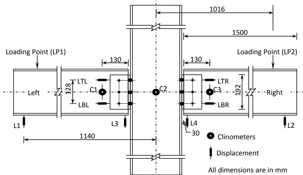
Fig. 3. Location of instrumentation in nominally pinned beam-to-column joint tests
