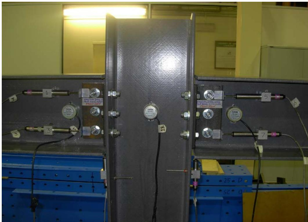
Fig. 5. Details of nominally pinned beam-to-column joint test Wmj254\_3M16\_ST1-3.
