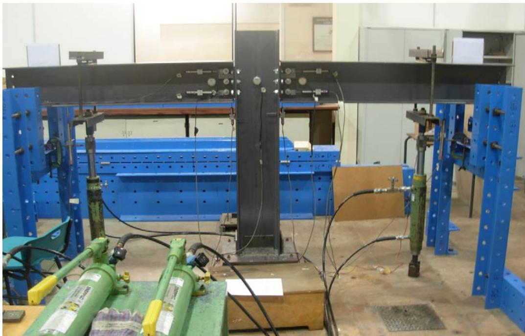
Fig. 2. General test arrangement for major-axis beam-to-column joint Wmj254\_3M16\_ST1-3.
