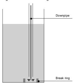
Figure 5: Examples of downward facing inlets with break ring
