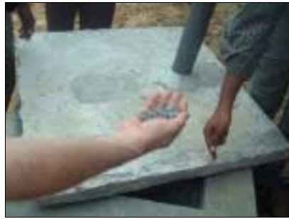
Filter media from a large gravel filter in Sri Lanka (Picture: B. Martinson)
