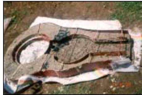
Mould developed in Ethiopia for making platters which reduced time to make a platter from 1 day to 1 hour
