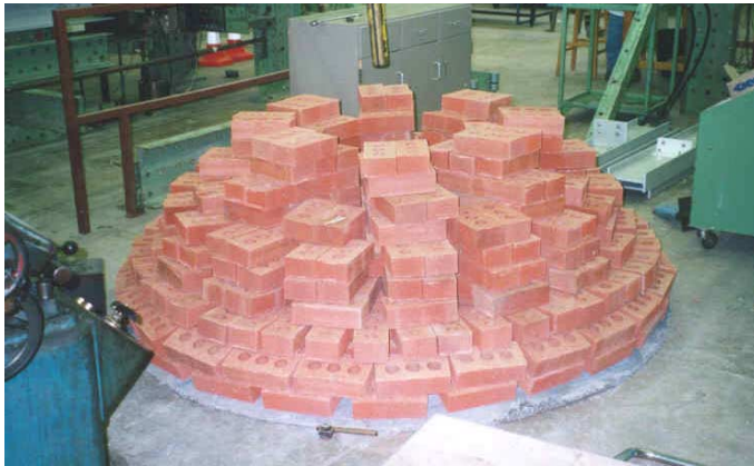
Figure 4 – Thin-shell cover under a load of 1000kg of bricks – an evenly distributed load
