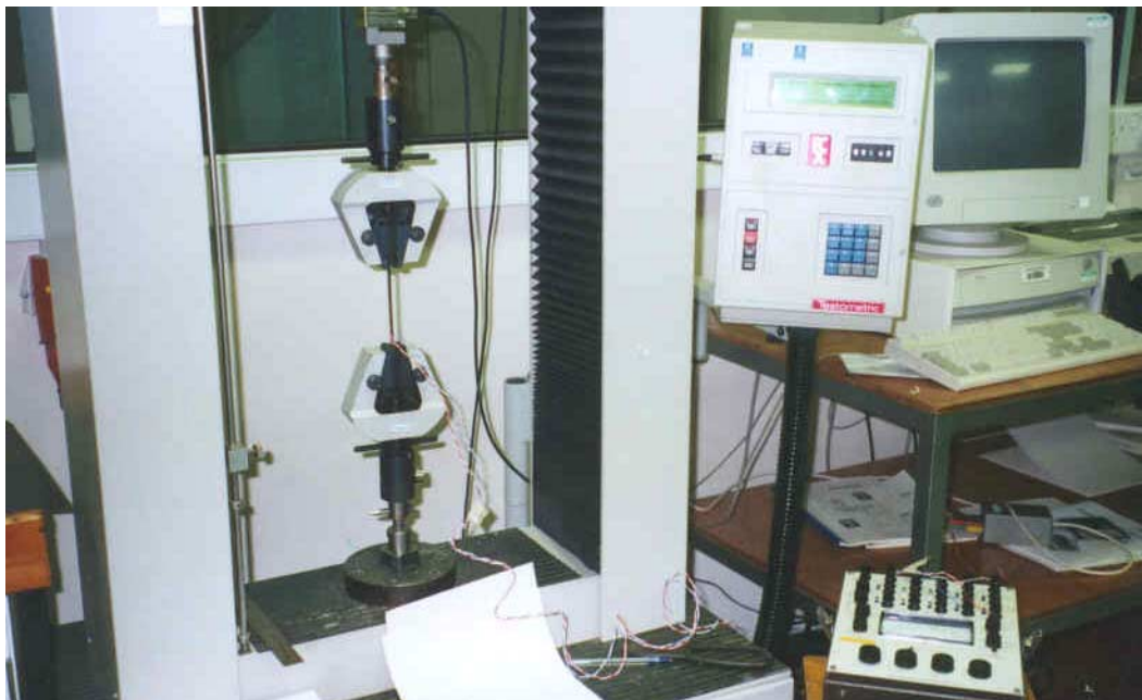
Figure 6 – Calibration of strain gauges using tensometer
