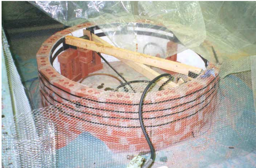
Figure 10 – Specimen under test, showing expansion ring
