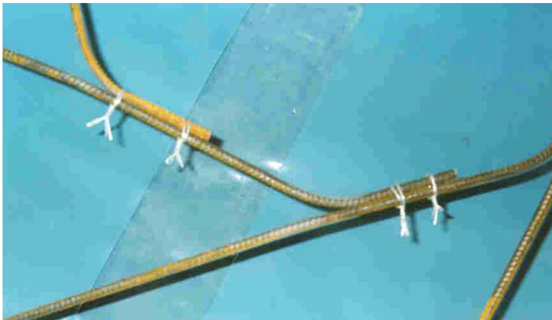
Figure 6. Arrangement for tying spokes to each other.
